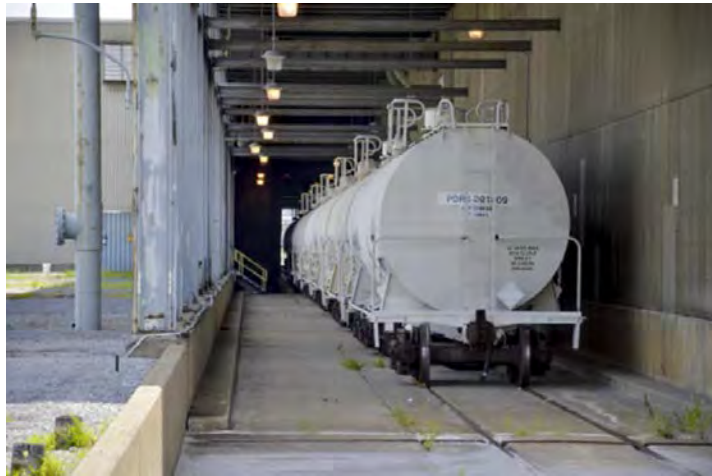
Figure 2.3 Railcars utilized for the storage of R-114 refrigerant.
